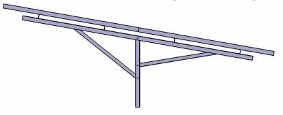
Structures made from roll formed steel profiles, that are hot dipped galvanized to 80 microns thickness 25 years warranty on structures Able to sustain wind loads of 150kmph Foundations can be reinforced concrete, ground screws, or rammed posts
